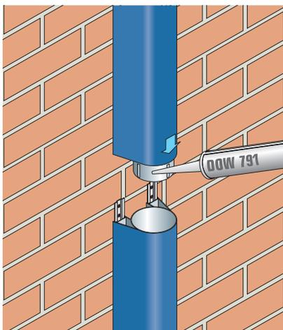
Pipe lengths are connected by sliding new pipe sections down over the fixing plates of the pipe below.
