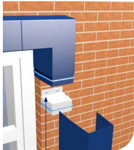
5. With all corners firmly in position, measure and cut the straight lengths to size.
