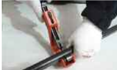
2. Cut pipe square to required length.
